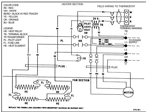
Figure 5 - Wiring Diagram
